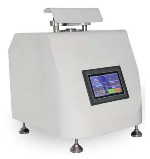
ZXQ-3 Automatic Metallographic Sample Mounting Press is used to mosaic small specimens, specimens in irregular shapes, or specimens which are not easy to take up-the preceding process before grinding and polishing metallographic or rock specimens.
